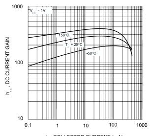
I , COLLECTOR CURRENT (mA) Fig. 4, DC Current Gain vs Collector Current
