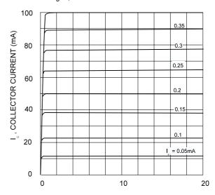
$V_{_{\circ}\,_{E}}$ , COLLECTOR-EMITTER VOLTAGE (V) Fig. 6, Typical Emitter-Collector Characteristics
