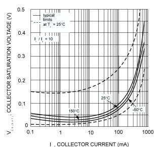
Fig. 3, Collector Sat. Voltage vs Collector Current
