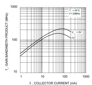
Fig. 2, Gain-Bandwidth Product vs Collector Current
