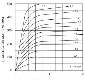
$V_{_{\circ}}$ , COLLECTOR-EMITTER VOLTAGE (V) Fig. 5, Typical Emitter-Collector Characteristics
