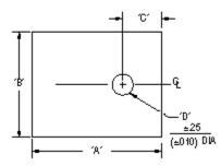
Thermasil III electrically insulating pad for a TO-220 device. Composed of a silicone elastomer binder with a thermally conductive filler and reinforced with finely woven glass cloth to resist tearing.
