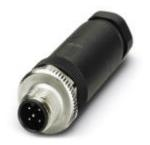
Connector, Universal, 5-position, Plug straight M12, A-coded, Screw connection, knurl material: Zinc die-cast, nickel-plated, cable gland Pg9, external cable diameter 6 mm ... 8 mm
