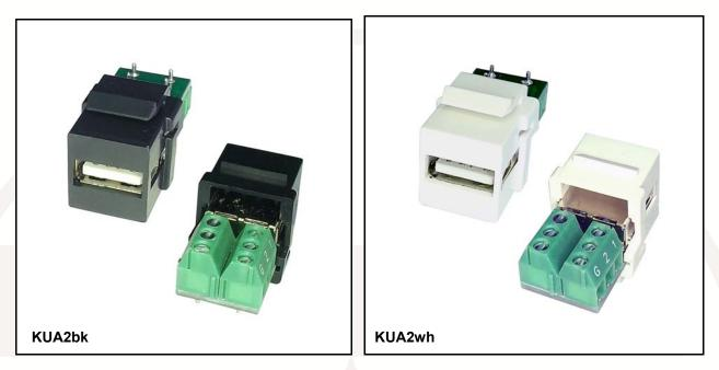
Suitable for field termination, repair and prototyping applications this 'DIY' socket enables an easy termination where a USB port is required. The 'breakout' board brings out all signal pins and the shield to screw-down terminal blocks for simple and reliable connection without the need for special tools.
