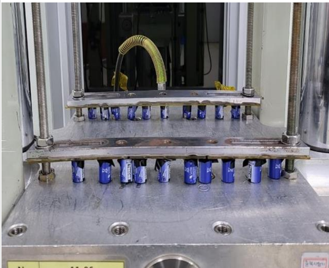
Photo.07 – Photographs of specimen before & after Shock test (Undischarged cells)
