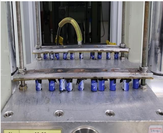
Photo.08 – Photographs of specimen before & after Shock test (Fully discharged cells)
