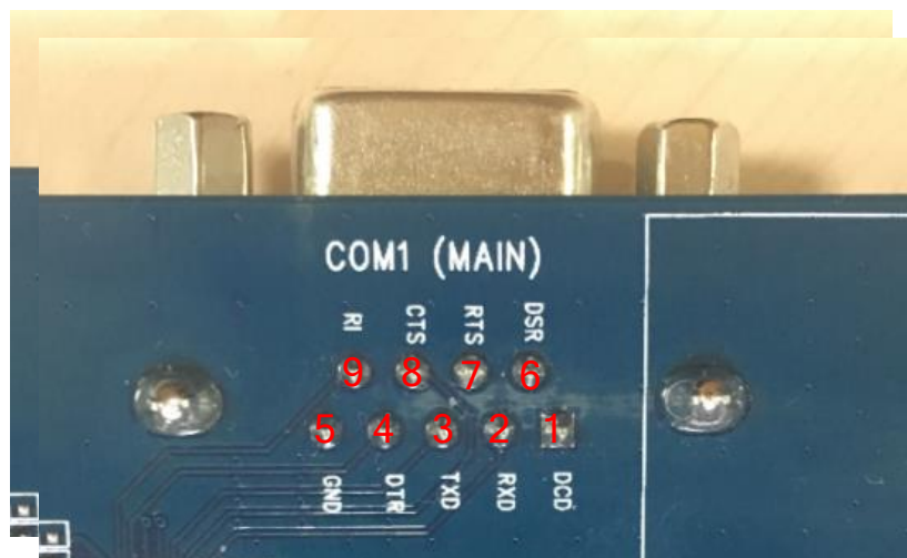
Figure 25: Pin Assignment of J401
