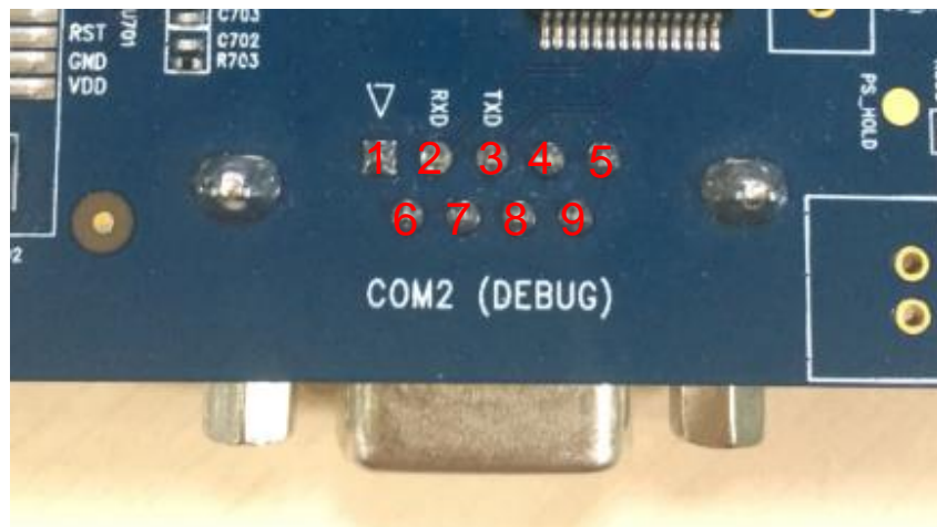
Figure 26: Pin Assignment of J402
