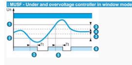
MUSF relays operate in window mode: they check that the controlled voltage stays between a minimum and maximum threshold.
