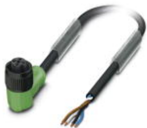
Sensor/Actuator cable, 4-position, PUR halogen-free, black-gray RAL 7021, free cable end, on Socket angled M12, A-coded, Cable length: 1.5 m, with plastic knurl
