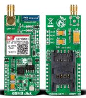
GSM3 click<sup>™</sup> carries **SIM800H**, a quad-band (**850/900/1800/1900MHz**) GSM/GPRS module that transmits voice, sms and data information. The board communicates with the target board MCU through the following mikroBUS<sup>™</sup> lines: Tx and Rx (UART), RST (reset), GP1 (status indicator), GP2 (RTS), GP3 (GPIO1), GP4 (PWRKEY, used to power on/off the module) and GP5 (CTS). GSM3 click<sup>™</sup> is designed to use 3.3V and 5V I/O voltage levels.
