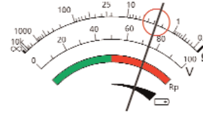
Figure 15: Resistance reading between 'X' and 'Y' terminals
