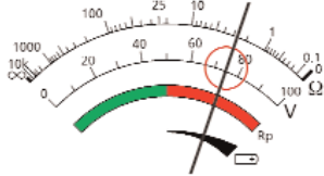
Figure 14: Analogue display indicating ground noise voltage measurement
