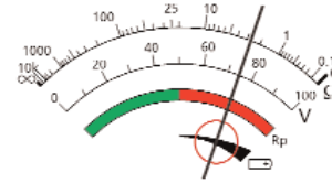
Figure 12: Analogue display indicating remaining battery life
