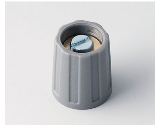
A2513048 ROUND KNOB 13.5, without line ABS (UL 94 HB) dusty grey RAL 7037 13x15mm 4mm
