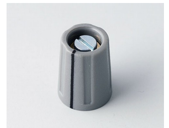
A2610038 ROUND KNOB 10, with line ABS (UL 94 HB) dusty grey RAL 7037 10x14mm 3mm
