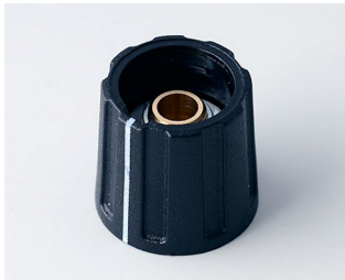
A2616060 ROUND KNOB 16, with line ABS (UL 94 HB) black RAL 9005 16x15mm 6mm
