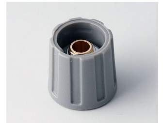
A2516068 ROUND KNOB 16, without line ABS (UL 94 HB) dusty grey RAL 7037 16x15mm 6mm
