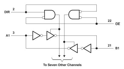
Figure 4. Logic Diagram (Positive Logic)
