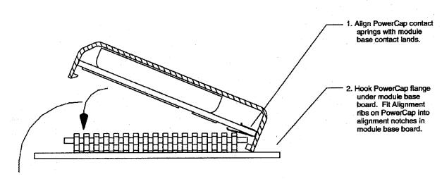
3. Push down slot side of PowerCap until it snaps onto module base.
