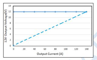
Figure 6. Current Limitation on  $V_1$  ( $V_i = 230 \text{ VAC}$ )
