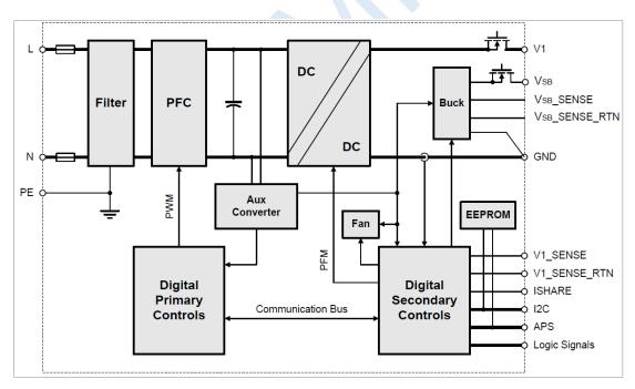
Figure 1. TET1500 Series Block Diagram
