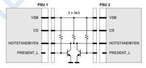
Figure 13. Recommended hot-standby configuration
