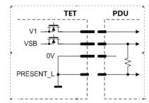
Figure 9. PRESENT\_L signal pin
