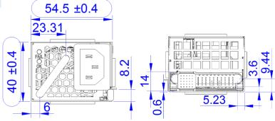
Figure 23. Front and Rear View
