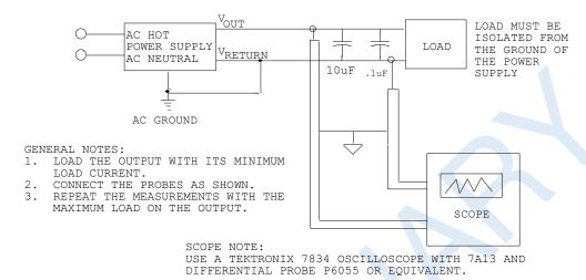
Figure 5. Output ripple test setup
