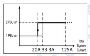
Figure 11. Hot-standby enable/disable current thresholds
