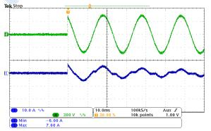
Figure 4. Inrush current, Vin = 305 VAC, 90°, CH1: Iin (10A/div), CH4: Vin (300V/div)
