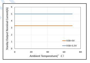
Figure 7. Current Limitation and Temperature Derating on 3.3 / 5 VsB
