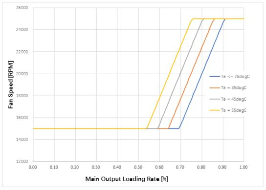
Figure 20. Fan speed VS main output load
