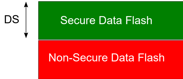
Figure 13-3. SAM L11 Data Flash Memory Mapping
