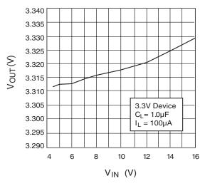
Figure 4. Output Voltage vs. Input Voltage
