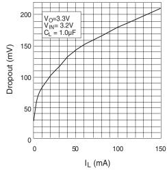
Figure 5. Dropout Voltage vs. Load Current
