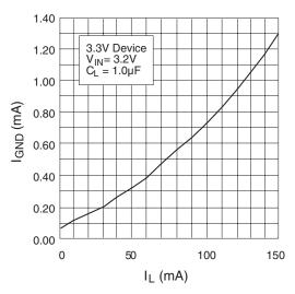
Figure 1. Ground Current vs. Load Current
