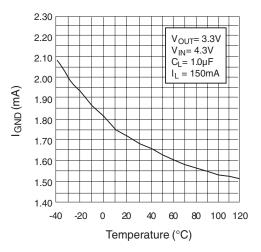
Figure 9. Ground Current in Dropout vs. Temperature
