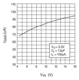
Figure 2. Ground Current vs. Input Voltage
