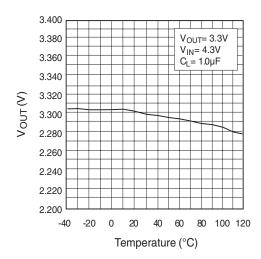
Figure 10. Output Voltage vs. Temperature
