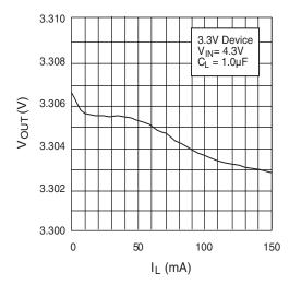
Figure 6. Output Voltage vs. Load Current
