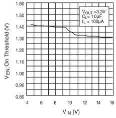
Figure 11. ENABLE Voltage, ON Threshold vs. Input Voltage
