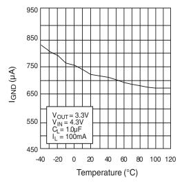
Figure 8. Ground Current vs. Temperature at  $I_{LOAD} = 100 \text{mA}$
