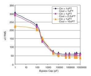
Figure 12. Output Noise vs. Bypass Capacitor Value
