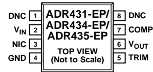
Figure 1. 8-Lead SOIC_N (R-8)
