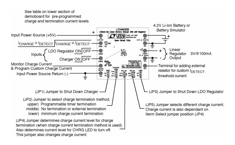
Figure 1. Proper Measurement Equipment Setup
