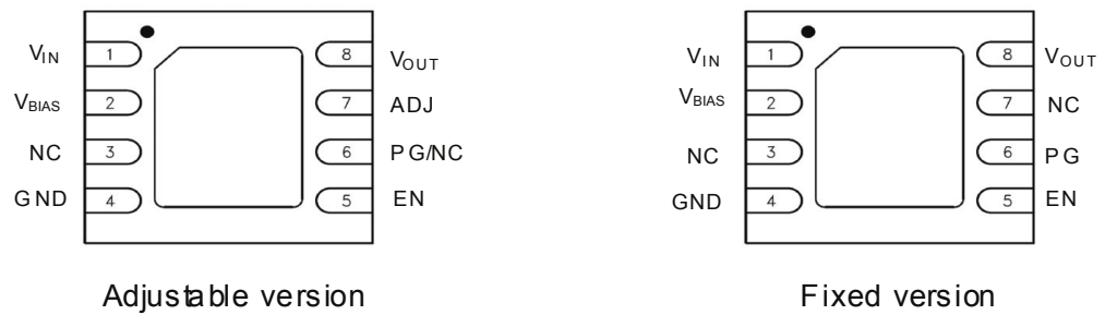
Figure 2. Pin connection (top view)
