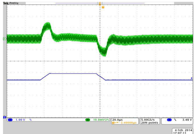
Figure 14. Line Transient, 200 mA Load, 10 μs Step
