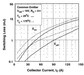
Figure 17. Switching Loss vs. Collector Current
