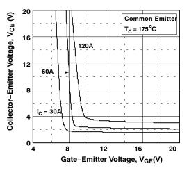
Figure 8. Saturation Voltage vs. V<sub>GE</sub>
