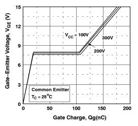
Figure 10. Gate Charge Characteristics
