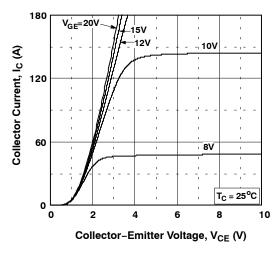
**Figure 1. Typical Output Characteristics**
