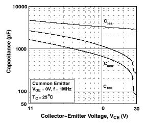
Figure 9. Capacitance Characteristics
