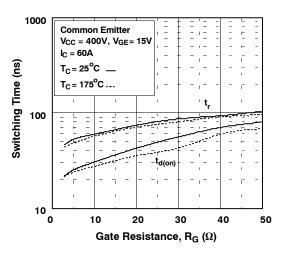
Figure 12. Turn-on Characteristics vs. Gate Resistance
