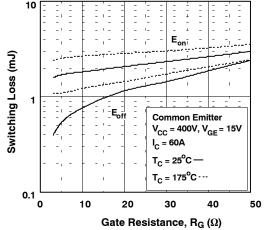
Figure 16. Switching Loss vs. Gate Resistance
