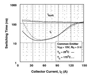
Figure 15. Turn-off Characteristics vs. Collector Current
