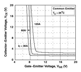
Figure 7. Saturation Voltage vs. V<sub>GE</sub>
