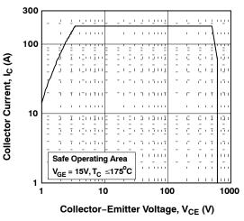
Figure 18. Turn Off Switching SOA Characteristics
