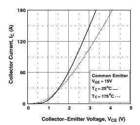
Figure 3. Typical Saturation Voltage Characteristics
