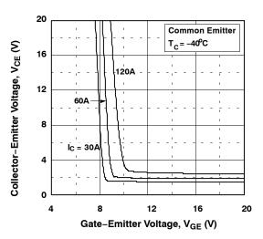
Figure 6. Saturation Voltage vs. V<sub>GE</sub>
