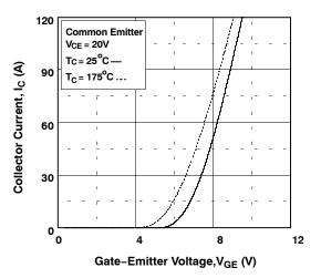
Figure 4. Transfer Characteristics
