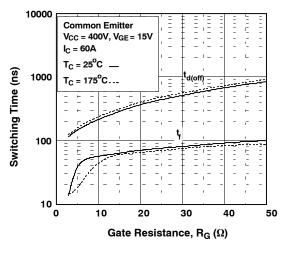
Figure 13. Turn-off Characteristics vs. Gate Resistance
