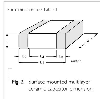
Fig. 2 Surface mounted multilayer ceramic capacitor dimension
