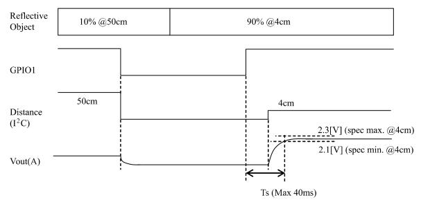
Response time of  $I^2C$  output is faster than that of Vout(A) because it is stabilized soon after distance data output. Distance data is updated every 20ms after response time.
