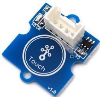
Grove - Touch Sensor enables you to replace press with touch. It can detect the change in capacitance when a finger is near by. That means no matter your finger directly touches the pad
