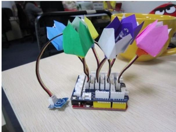
Connect the buds and the touch sensor onto the Grove Base Shield with the 10cm Grove cable. And then upload the code to your controller.
