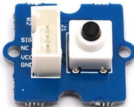
This new version of button Grove module contains one independent button, which are configured with pull-down resistor – ready for use with our microcontrollers as digital input. The button signals the SIG wire,NC is not used on this Grove module.
