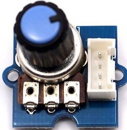
The potentiometer Grove produces analog output between 0 and VCC. The angular range is 300 degrees with a linear change in value. The resistance value is 10k ohms, perfect for Arduino use. This may also be known as a “rotary angle sensor” .
