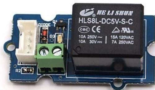
Relay is a useful tool to magnify your Arduino's control ability! Feed the control signal through the Grove interface, and relay will control the open/close of the external circuit that connected to the screw terminals. The
