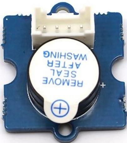
This is a simple yet enjoyable Grove to use. The piezo can be connected to digital outputs, and will emit a tone when the output is high. Alternatively it can be connected to an analog pulse-width modulation output to generate various tones and effects.
