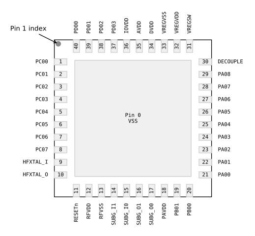
Figure 6.2. QFN40 Device Pinout
