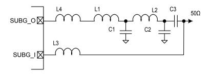
Figure 5.6. Typical 470 MHz Band RF impedance-matching network circuit
