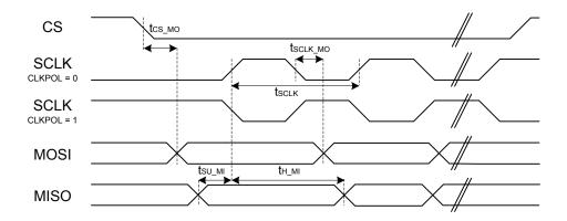
Figure 4.5. SPI Main Timing
