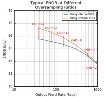
Figure 4.11. Typical ENOB vs. Oversampling Ratio
