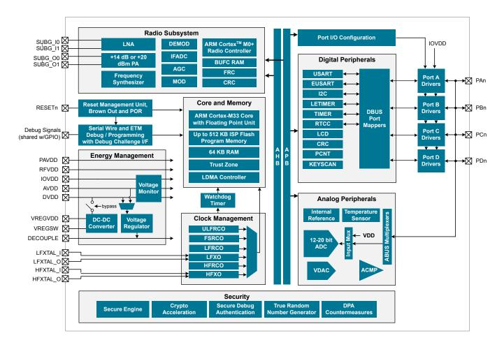
Figure 3.1. Detailed EFR32FG23 Block Diagram
