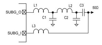
Figure 5.7. Typical 433 MHz Band RF impedance-matching network circuit
