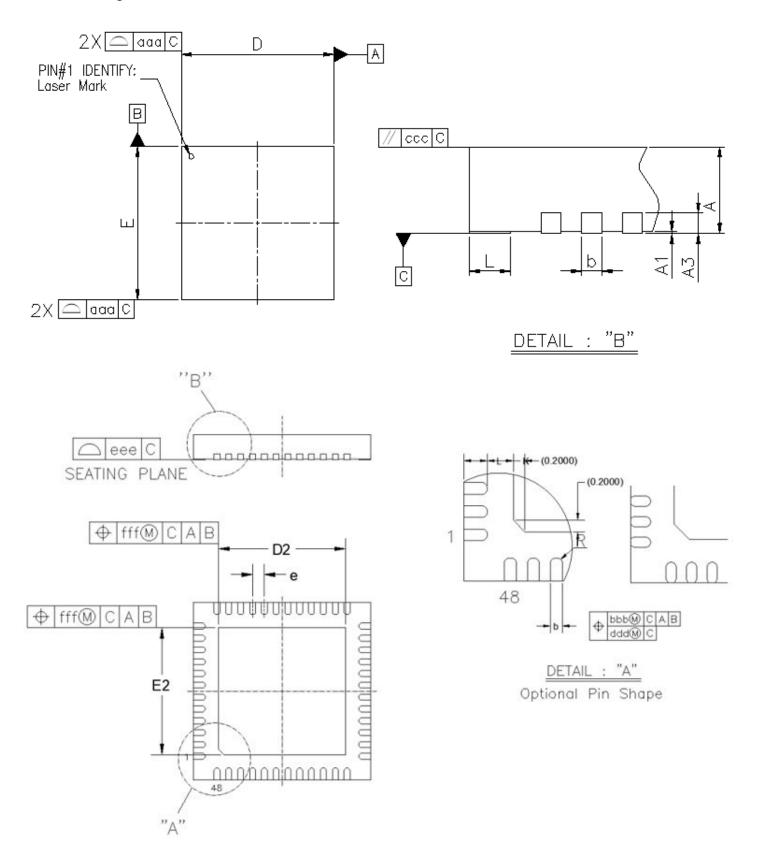
Figure 8.1. QFN48 Package Drawing
