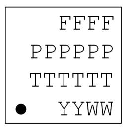
Figure 8.3. QFN48 Package Marking
