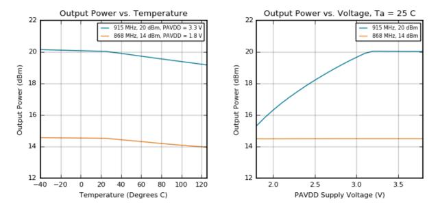
Figure 4.9. Transmitter Output Power
