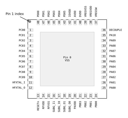
Figure 6.1. QFN48 Device Pinout
