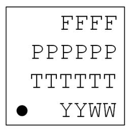
Figure 7.3. QFN40 Package Marking
