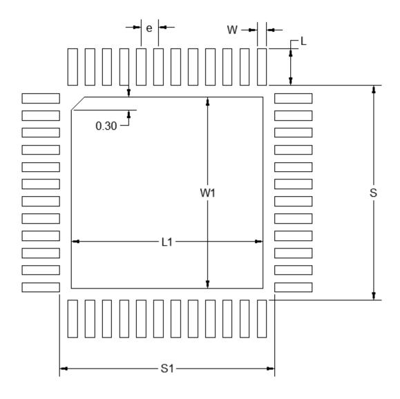
Figure 8.2. QFN48 PCB Land Pattern Drawing
