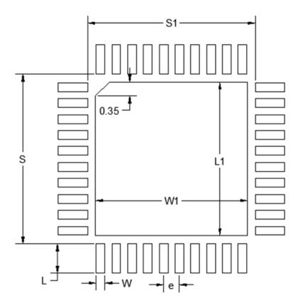
Figure 7.2. QFN40 PCB Land Pattern Drawing
