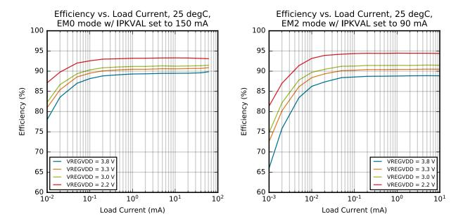
Figure 4.10. DC-DC Efficiency
