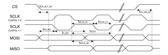
Figure 4.6. SPI Secondary Timing
