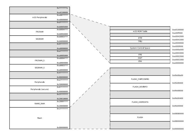
Figure 3.2. EFR32FG23 Memory Map — Core Peripherals and Code Space
