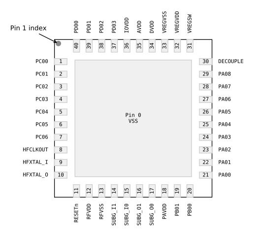
Figure 6.3. QFN40 with HFCLKOUT Device Pinout
