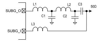
Figure 5.8. Typical 315 MHz Band RF impedance-matching network circuit
