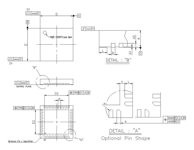
Figure 7.1. QFN40 Package Drawing
