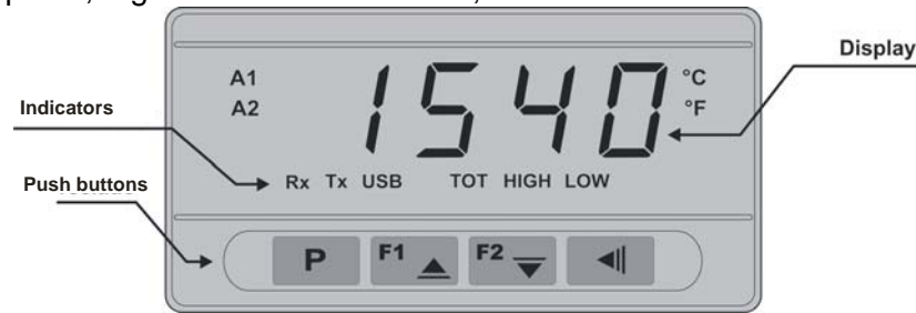
Figure 02: Identification of the front panel parts.
