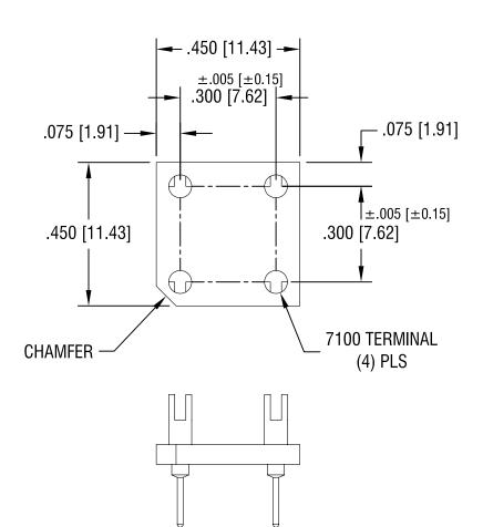
NOTE: **KEYSTONE ELECTRONICS CORP.** 1. BOARD MAT'L- .062 [1.57] G10 GLASS EPOXY www.keyelco.com • ASTORIA, N.Y. 11105-2017 • Tel (718) 956-8900 PART NAME 2. FORK TERMINAL MAT'L- BRASS, GOLD PLATE COMPONENT CARRIER BOARD MATERIAL AS NOTED DRN BY FINISH DATE BOONE 3.16.84 AS NOTED APP'D SCALE LN ЗX REDRAWN 7.15.08 А TOLERANCES INCH [MM] CODE DWG NO. ±.010 [±0.25] DECIMAL 7111 ANGULAR  $\pm 1^{\circ}$ С
