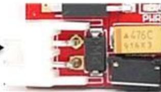
This connects to the main power source for the Seeeduino Mega (Vin) ranges from 6 – 20 Volts, keep in mind that this voltage input is polarity sensitive
