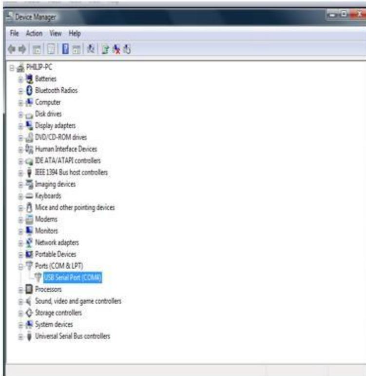
\*After the driver installation, go to **My Computer > Properties > Device Manager** then look for **Ports (COM and LPT) > USB Serial Port (COMn)** the n may vary from one PC to another, in this case we have 4. Take note of this since it will be used in the Arduino IDE configuration.
