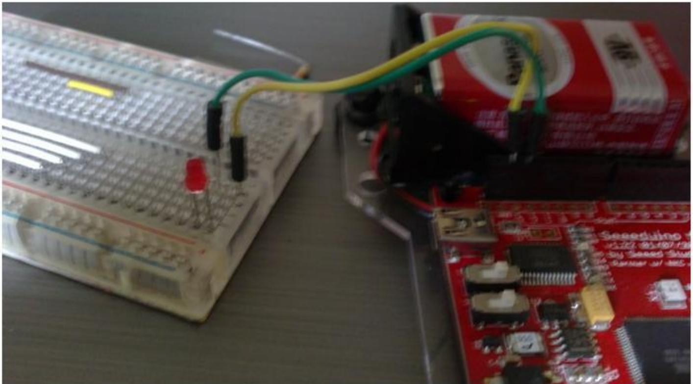
Green is Pin13 while Yellow in Ground, in this set up I used a 3.5mm LED the maximum current that should be forced to it must be below 10mA. However to have a brighter blink I omitted the series resistor - thus in order to dim the output just add a resistor in series of the LED. Also take note that an LED's legs can't be and shouldn't be interchanged. See [http://en.wikipedia.org/wiki/Light-emitting\\_diode](http://en.wikipedia.org/wiki/Light-emitting_diode) for more details.
