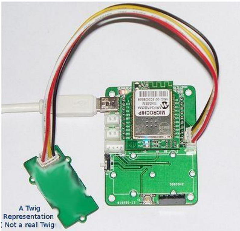
Grove - XBee Carrier - Connected to Wifi Bee and Powered By USB
