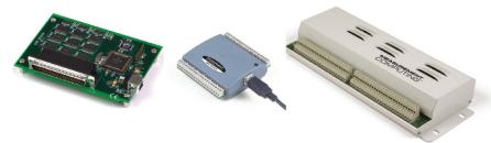
USB-DIO24 Series boards (left) provide 24 DIO. The USB-1024 Series (middle) provide the same functionality as the USB-DIO24 Series and are shipped in a case. USB-DIO96H Series (right) provide 96 DIO, high-drive current output and are shipped in a metal enclosure.
