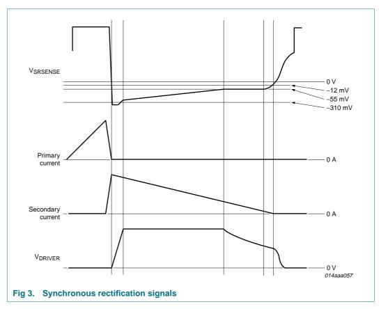
If the secondary stroke of the flyback converter is shorter than 2  $\mu$ s (typical), the driver output is disabled. This will guarantee stable operation for very low duty cycles. When the secondary stroke increases above 2.2  $\mu$ s (typical) then the driver output is again enabled.
