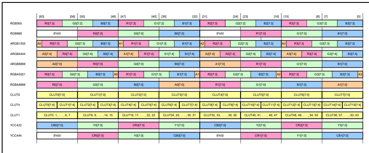
Figure 35.4 Data Arrangement with Endian Control Disabled (GR_RDSWA = 000)
