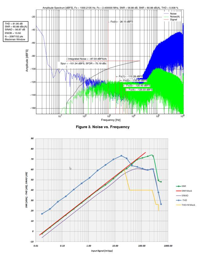
Figure 4. THD, SINDA, and SNR vs. Input Amplitude
