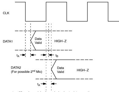
t<sub>A</sub> – Microphone delay from clock edge to data assertion.
