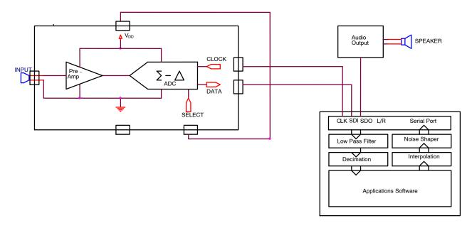
Figure 7. Mono Microphone Application Circuit
