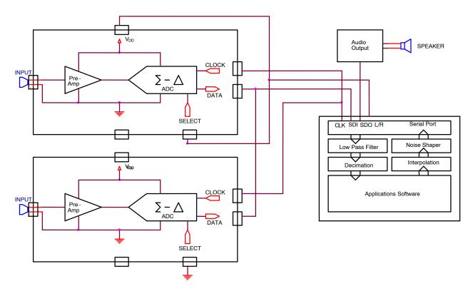
Figure 8. Stereo Microphone Application Circuit
