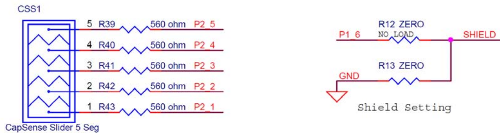
Figure 5-13. Schematics and Board Highlight of CapSense Slider and Shield Setting
