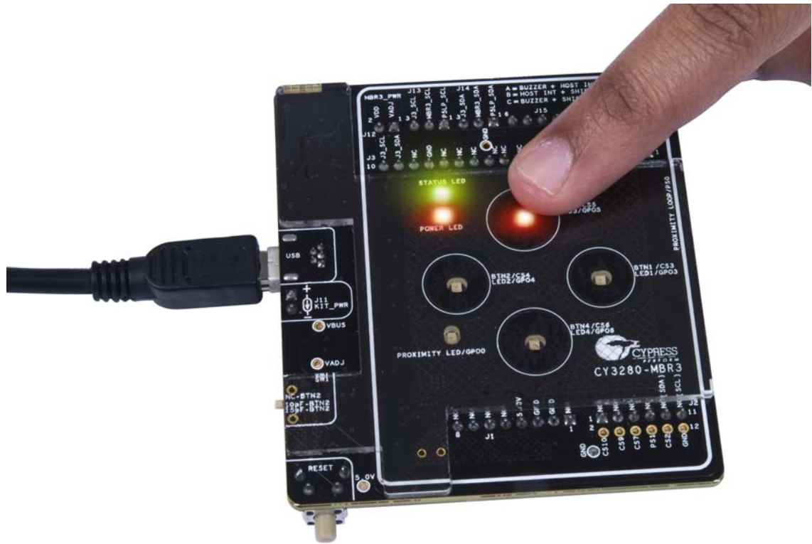
Figure 5-16. Auto-Reset Feature - LED Output Five Seconds After Button Touch
