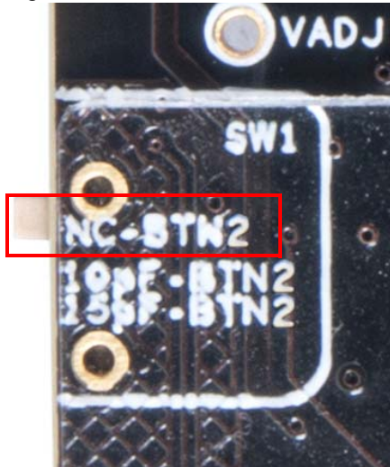
Figure 3-19. SW1 Slide Switch in NC-BTN2 Position
