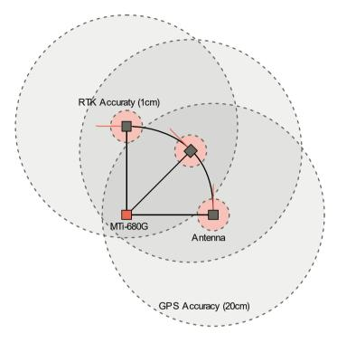
Figure 5: Lever arm correction for MTi-680G
