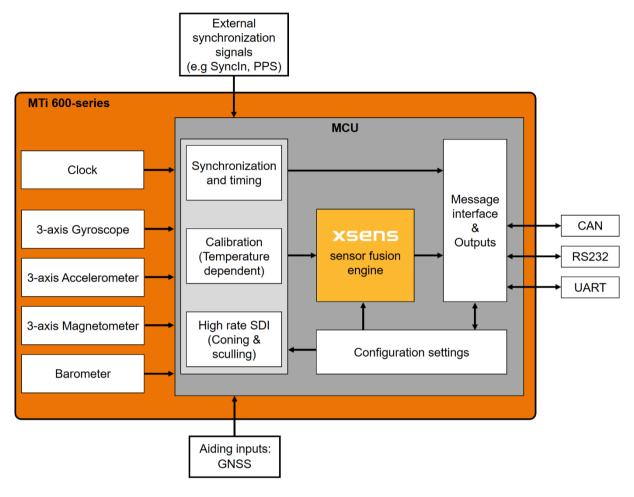
Figure 1: MTi 600-series module diagram
