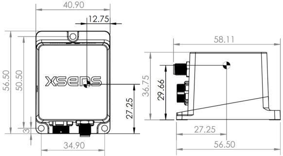
Figure 9: Location origin of measurements MTi-680G (dimensions in mm)
