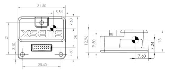
Figure 8: Location origin of measurements MTi-600 module (dimensions in mm)
