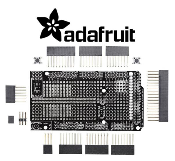
This is an extra-large proto-shield, specifically designed for the Mega! It comes with PCB, two buttons and a full set of stacking headers. You can stack this shield easily since it comes with extra-long female headers.
