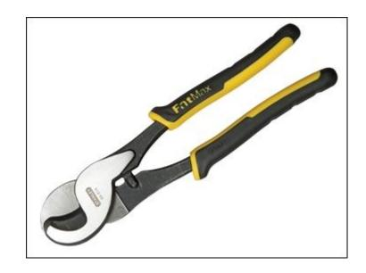
The FatMax cable cutter is ideal for cutting lengths of thick cable and has the following features: bimaterial handles, heat treated chrome steel forging, interlocking joint assembly, slim line design and high frequency heat treated cutting edges.
