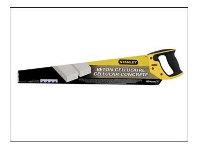
The FatMax concrete saw has a specially designed 660mm (26 in) blade which is ideal for cutting cellular blocks and soft stone. The teeth are induction hardened and the comfortable bi-material handle is screwed and ultrasonically welded. the handle is marked with 45° and 90° angles and the blade has 1.4 teeth per inch.
