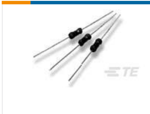
TE Part #6-1625892-1 3W SM M/OX 5% 5K6
