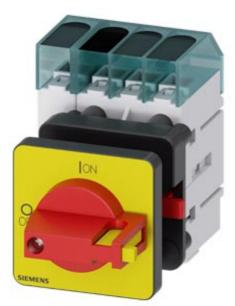
Load disconnector 3LD3, lu 16 A Main switch 3-pole + N Rated operating capacity at AC-23 A at 400V 7.5kW Front plate mounting Basic switch with Central hole mounting 22.5mm Toggle drive red / yellow 48x48 mm
