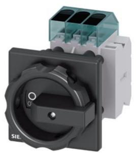
Load disconnector 3LD3, Iu 16 A Main switch 3-pole Rated operating capacity at AC-23 A at 400V 7.5kW Front plate mounting Basic switch with Central hole mounting 22.5mm Rotating drive black 66 x 66 mm with auxiliary switch 1OE + 1S
