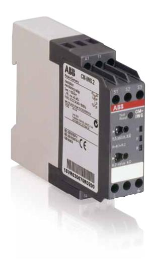
The CM-IWS.2 is used to monitor insulation resistance in accordance with IEC 61557-8 in pure IT AC systems. Measured are insulation resistances between system lines and system earth. When falling below the adjustable threshold values, the output relays switch into the fault state.
