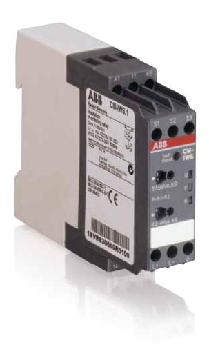
The CM-IWS.1 and CM-IWN.1 serve to monitor insulation resistance in accordance with IEC 61557-8 in unearthed IT AC or DC systems. Measured are insulation resistances between system lines and system earth. When falling below the adjustable threshold values, the output relays switch into the fault state. With CM-IWS.1 und CM-IWN.1 a pulsating measuring signal is fed into the system to be monitored and the insulation resistance calculated.
