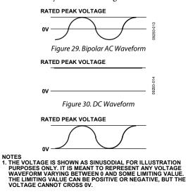
Figure 31. Unipolar AC Waveform
