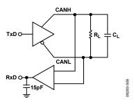
Figure 24. Switching Characteristics Measurements
