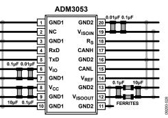
Figure 28. Recommended PCB Layout
