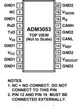
Figure 4. Pin Configuration
