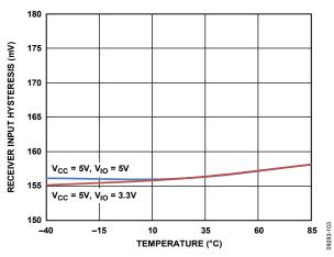
Figure 8. Receiver Input Hysteresis vs. Temperature
