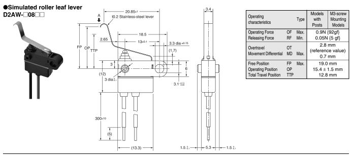
Note1. Unless otherwise specified, a tolerance of  $\pm 0.2$  mm applies to all dimensions.
