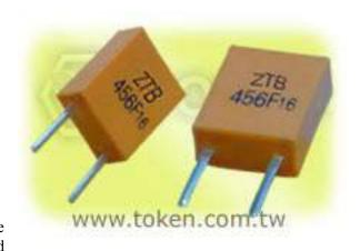
to provide frequency modulation for HI-FI automobile stereo application. The ZTB 500/503F Series is designed for TV horizontal synthesizer circuits. These Ceramic Resonators are offered in the following frequency accuracy with applicable IC. All ZTB456/500/503/912F are Murata Compatible CSB456/503/912F.
