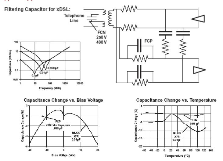
The capacitance of SMT film chips is much more stable with applied voltage and with changes in temperature than multilayer ceramic capacitors. Add in the low ESR characteristics of film chips and the final result is improved performance in filter circuit applications.
