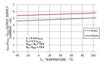
Figure 10: I<sub>SS2H</sub>/I<sub>SS2L</sub> vs. Temperature
