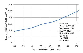
Figure 19:  $t_{OC(RESET)}/t_{OC(MUTE)}$  vs. Temperature
