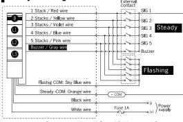
Do not connect the power line and flashing or steady lines
