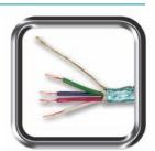
Van Damme Brown Series Ecoflex is a foil screened Low Smoke Zero Halogen (LSZH) single quad and starquad multicore primarily for the installation market. As this cable is specified for installation a foil screen as opposed to braided copper is used as the cable should not have to cope with dynamic flexing.
